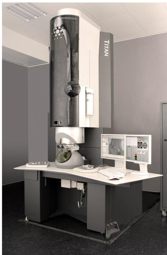
Figure 1: FEI Titan 80-300 transmission electron microscope (photograph by courtesy of Ralf-Uwe Limbach (Forschungszentrum Jülich)).
