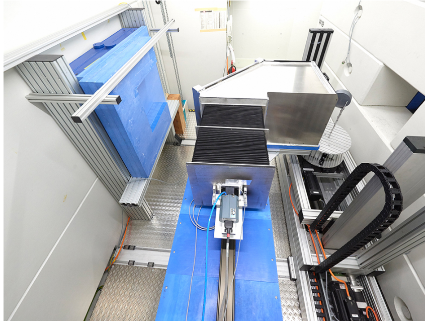
Figure 1: Instrument NECTAR: The fission neutrons are coming from the right, penetrating the sample fixed on the manipulator, and are detected by a CCD-based system (center). A beamstop (left) minimizes scattered radiation. (Copyright by W. Schürmann, TUM).
