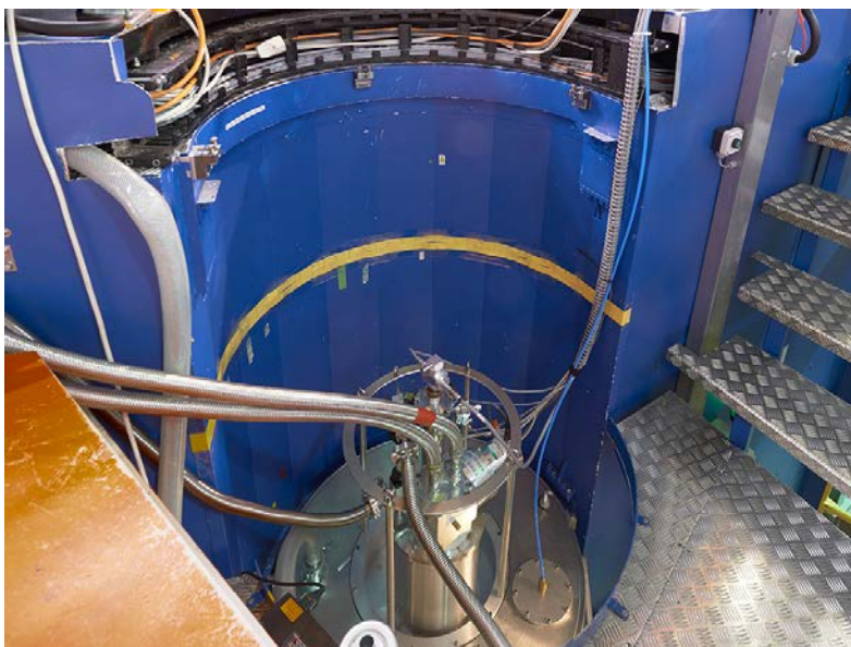
Figure 1: Top view of the CCR Cryostat inserted into the TOFTOF sample chamber. The blue panelling visible is the exterior of the detector housing (Copyright by W. Schürmann, TUM).
