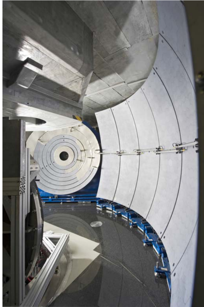
Figure 1: View inside SPHERES: the large array of Si(111) analyzer crystals covers a solid angle of about 2.5, which is 20 % of 4\pi (Copyright by A. Heddergott, TUM).
