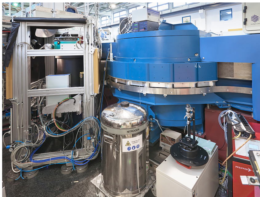
Figure 1: Instrument BIODIFF with the detector unit on the left side, monochromator shielding (blue) on the right side (Copyright by W. Schürmann, TUM).
