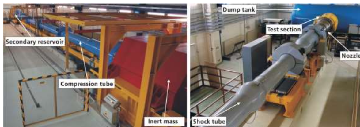
Figure 3: Photographic views of the High Enthalpy Shock Tunnel Göttingen, HEG.
