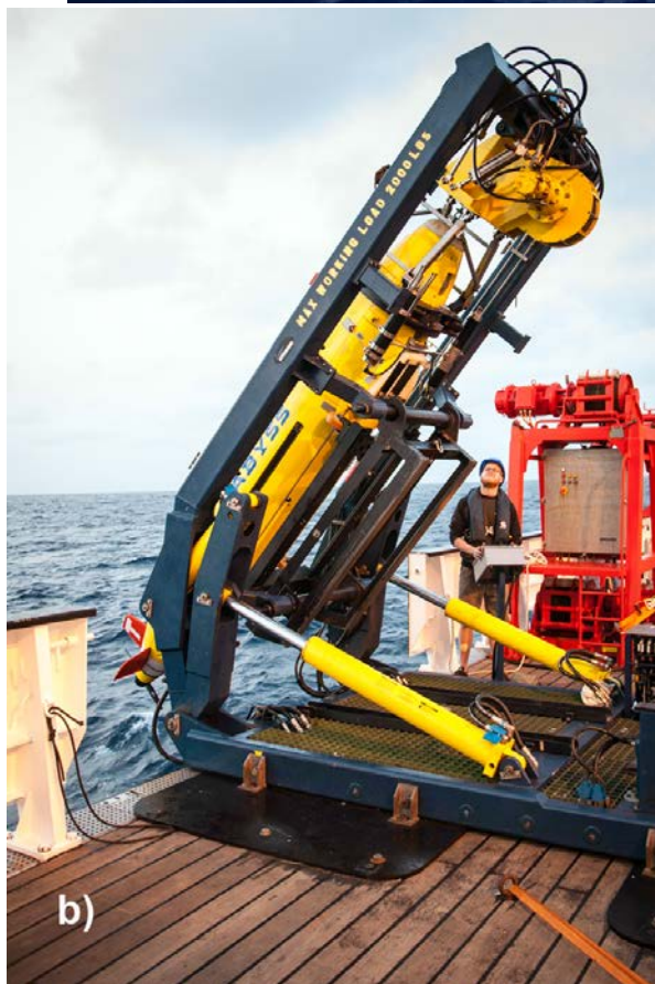
Figure 1: AUV “ABYSS“, a) at the sea surface approaching the German research vessel “POSEIDON” for recovery, b) deployed with its launch and recovery system, c) novel LED flash system in the front and the camera behind a dome port in the tail section of the vehicle.
