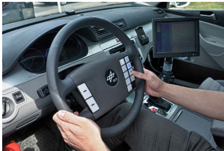
Figure 5: Steering wheel of FASCar ® -II.
