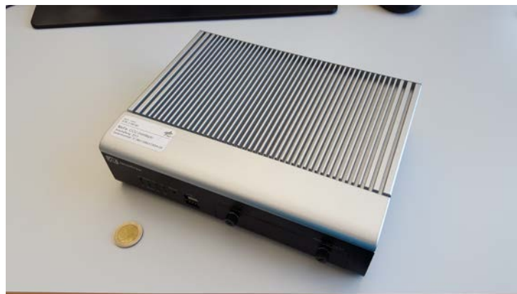
Figure 1: V2X communication unit.
