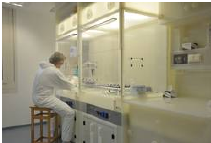
Figure 1: HELGES clean laboratory facilities showing metal-free laminar workstations.
