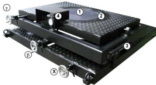
Figure 3: General purpose adapter available for sensor mounting. ① Opening for sensor baffle (covered); ② Flanges of different size to mount sensor; ③ Sliding rule to read the X setting; ④ Meters to read the settings of \beta and \gamma ; \textcircled{X} , \textcircled{\beta} , \textcircled{\gamma} : Hand wheels to align the indicated axes.
