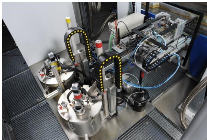
Figure 9: Two-component injection unit with automated docking system.
