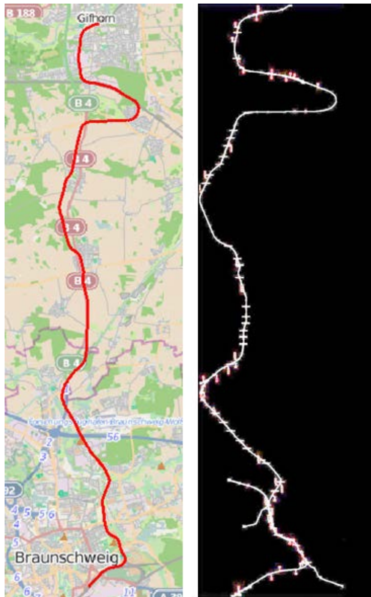
Figure 2: Virtual railway reference track as overlay on OSM (left), with signals and crossings (right).
