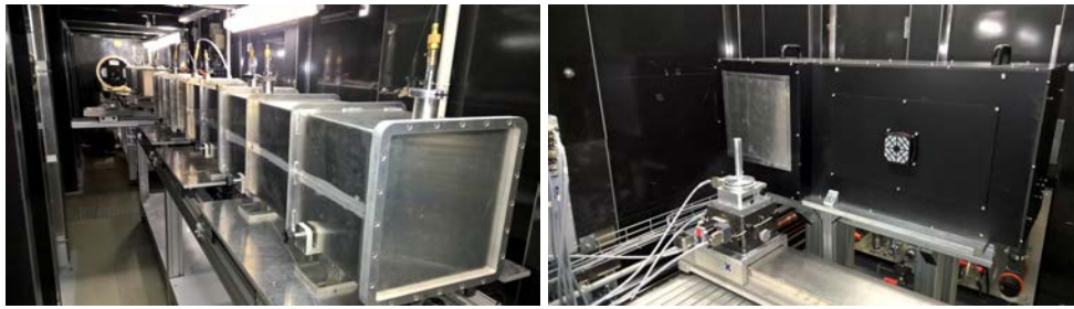
Figure 1: View of V7. Flight path equipped with containers filled with He gas for loss free transport of the neutron beam to the sample position (left). Sample position equipped with translation, tilt and rotation stages. The detector box with active area of 30 cm x 30 cm is behind the sample stage (right).
