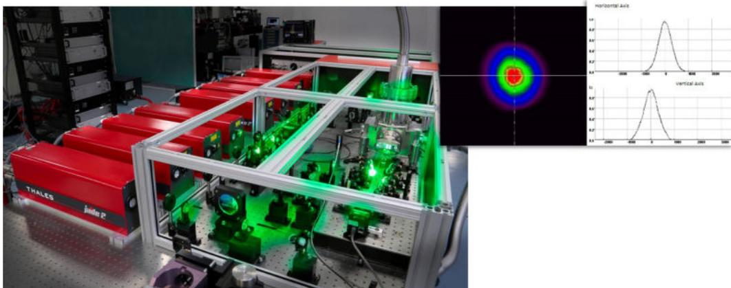
Figure 5: The block of eight pump lasers and the second amplification stage. The first pump laser is used to pump the first amplification stage, while the remaining seven pump lasers are employed for pumping the cryo-cooled Ti:Sapphire crystal of the second amplification stage. The typical beam profile of a Jade 2 pump laser is shown on the right.
