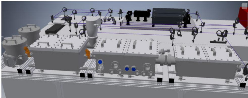
Figure 7: HHG beamline for high-energy photon and electron scattering experiments. From right to left: focusing chamber, HHG source chamber containing the gas cell, monochromator, and experiment and detection chambers. The high-energy photon beam is generated and guided inside vacuum to avoid scattering in air.
