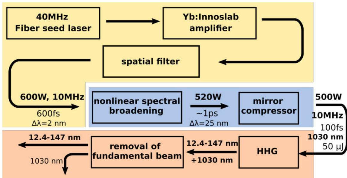
Figure 10: Schematic setup of  $\mu$ SPARC\_SIRIUS for spin- and time-resolved electron momentum microscopy, which consist of Innoslab amplifier (shaded yellow region) (Russbueltd et al., 2015), nonlinear compression using multi-pass cell (Weitenberg et al., 2017) (shaded blue region) and XUV-initiated HHG (shaded orange region).
